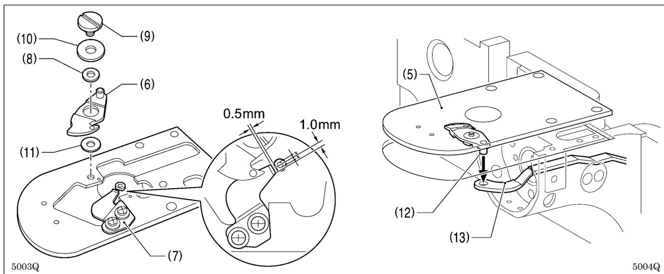
4. Install the new fixed knife (7) in the position shown in the illustration.
