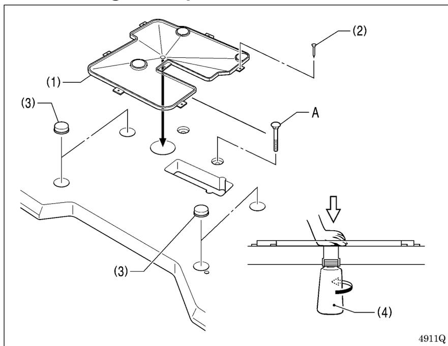
For motor-driven work clamp specifications, install the treadle unit mounting bolt (A) before installing the oil pan.
