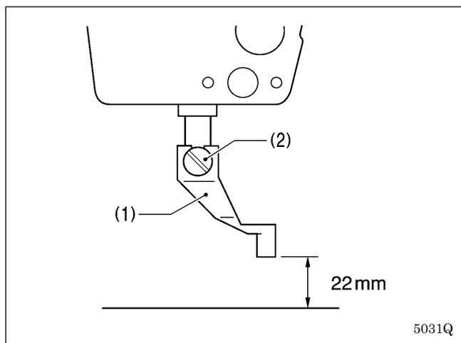
Install the presser foot (1) with the screw (2) so that the distance from the bottom of the presser foot to the top of the needle plate is 22 mm when the sewing machine is stopped and the presser foot (1) is raised.
