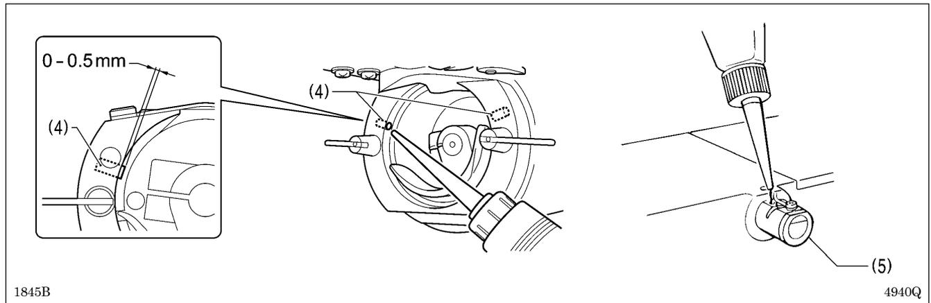
3. Pour oil in through the two holes of the shuttle race base assembly so that the felt (4) is lightly moistened.
