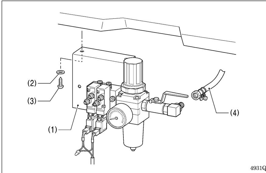
Install underneath the work table.
