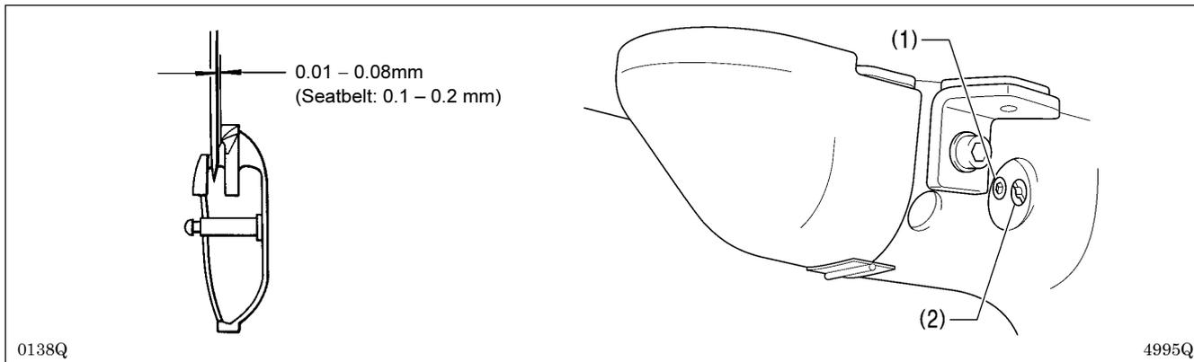
Turn the machine pulley to align the tip of the rotary hook with the center of the needle, and then loosen the set screw (1) and turn the eccentric shaft (2) to adjust so that the clearance between the needle and the rotary hook is 0.01 – 0.08 mm.
