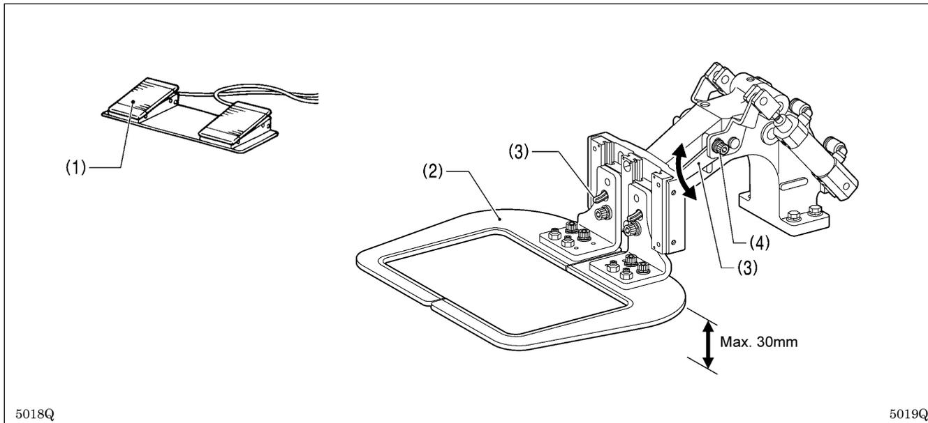
1. Turn on the air, and depress the work clamp switch (1) to raise the work clamp (2).
