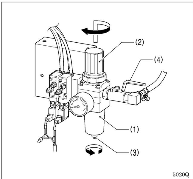
Lift up the handle (2) of the regulator (1) and then turn it to adjust the air pressure to 0.5 MPa. After adjustment is complete, push the handle (2) downward to lock it.
