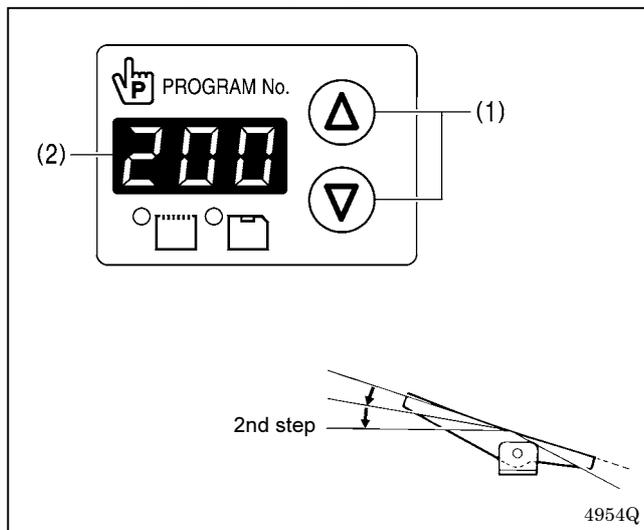
1. Press the  $\Delta$  or  $\nabla$  key (1) to select the program number that is loaded into the internal memory.
