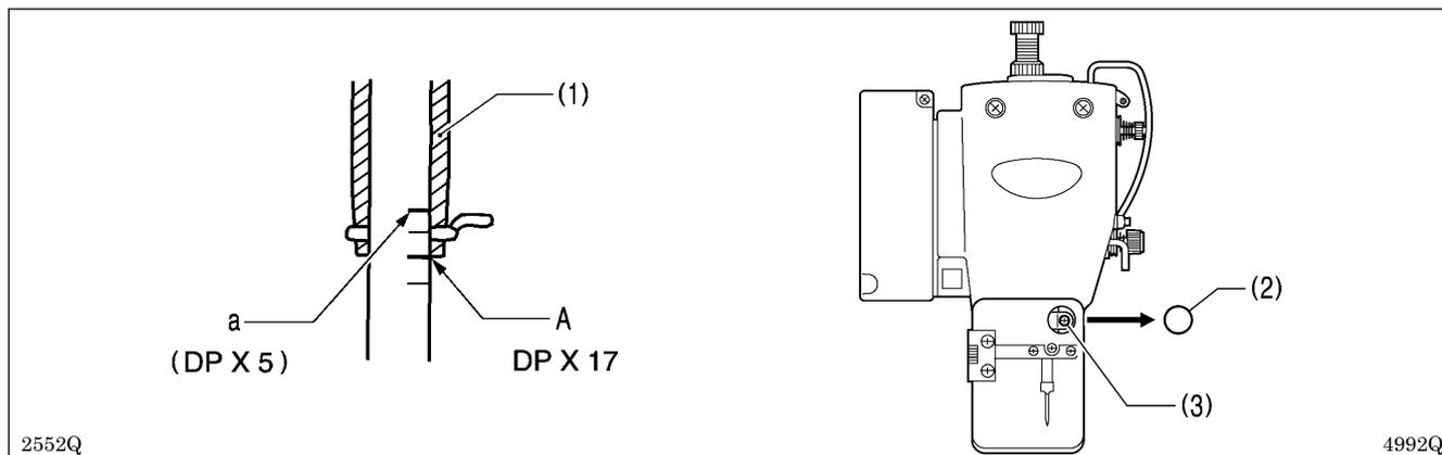
Turn the machine pulley to move the needle bar to the lowest position. Then remove the rubber plug (2), loosen the screw (3) and then move the needle bar up or down to adjust so that the second reference line from the bottom of the needle bar (reference line A) is aligned with the lower edge of the needle bar bush (1).
