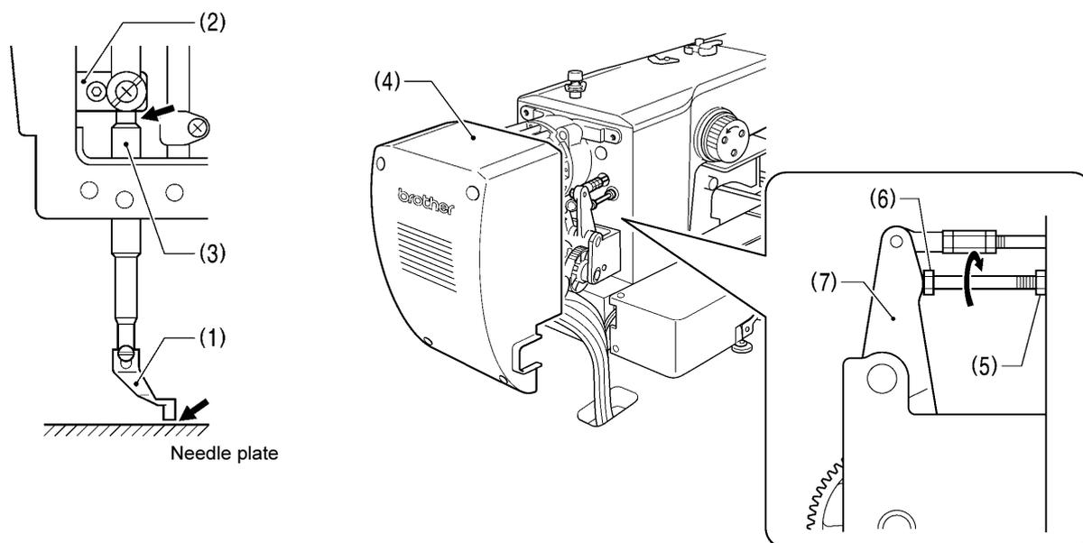
1. With the intermittent presser foot (1) lowered, turn the pulley to move the intermittent presser foot (1) to its lowest position.
