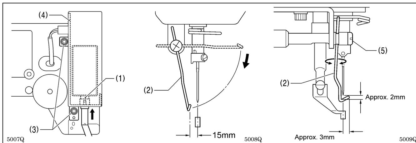
1. Loosen the two screws (3) and shift the entire solenoid setting plate (4) up or down to adjust so that the thread wiper (2) is 15 mm in front of the needle center when the plunger (1) of the thread wiper solenoid is driven to the full stroke.
