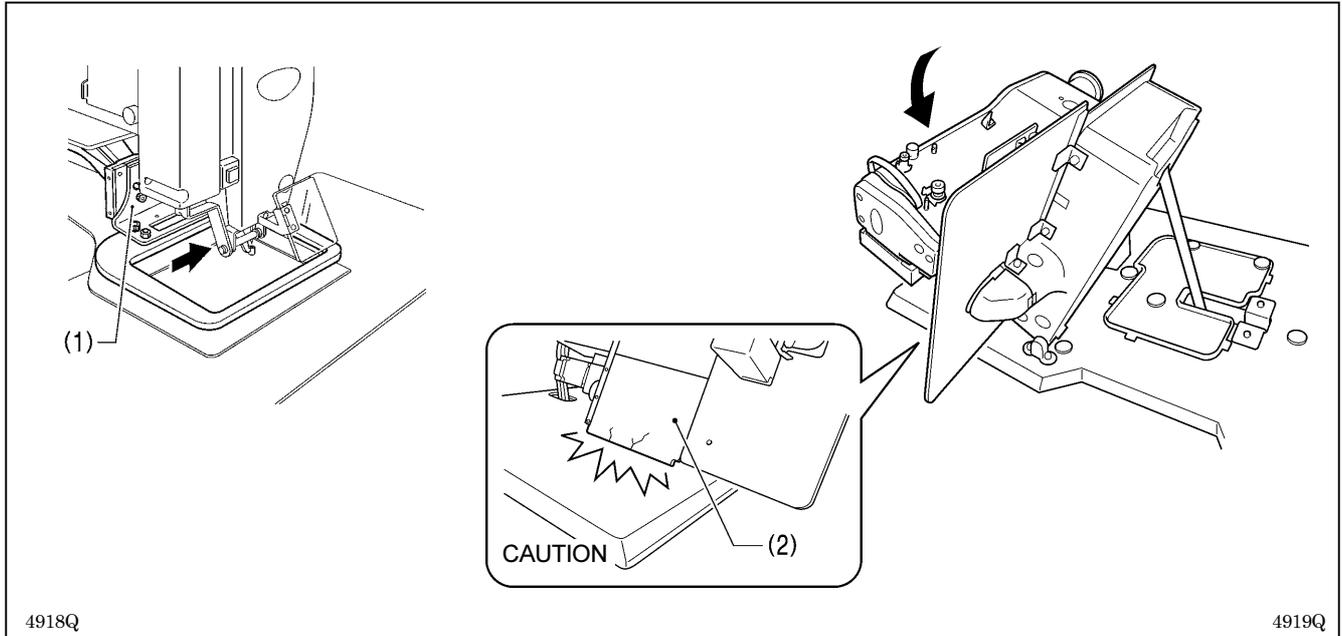
1. Move the presser arm assembly (1) as far as it will go in the direction of the arrow in the illustration (to the right when looking from the front of the sewing machine).
