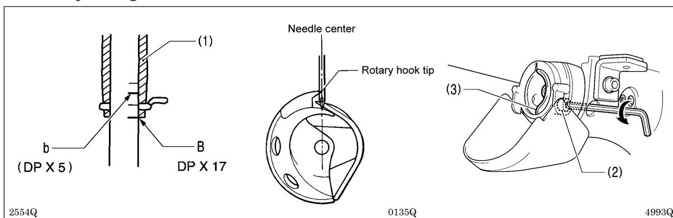
Turn the machine pulley to raise the needle bar from the lowest position until the lowest reference line on the needle bar (reference line B) is aligned with the lower edge of the needle bar bush (1), and then loosen the bolt (2) and move the driver (3) so that the tip of the rotary hook is aligned with the center of the needle.
