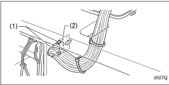
5. Close the cord presser plate (2) in the direction of the left arrow, and secure it by tightening the two screws (1).
