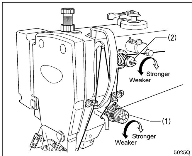
1. Turn the tension nut (1) (main tension) to adjust the tension as appropriate for the material being sewn.
