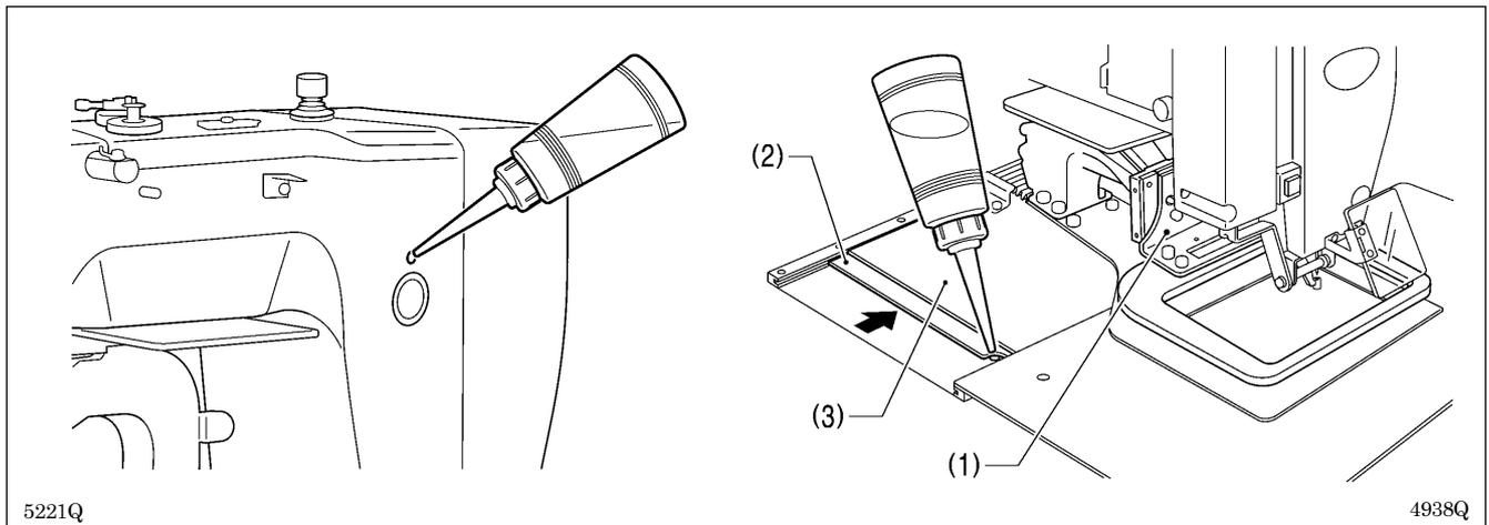
1. Fill the arm-side oil tank with oil.
