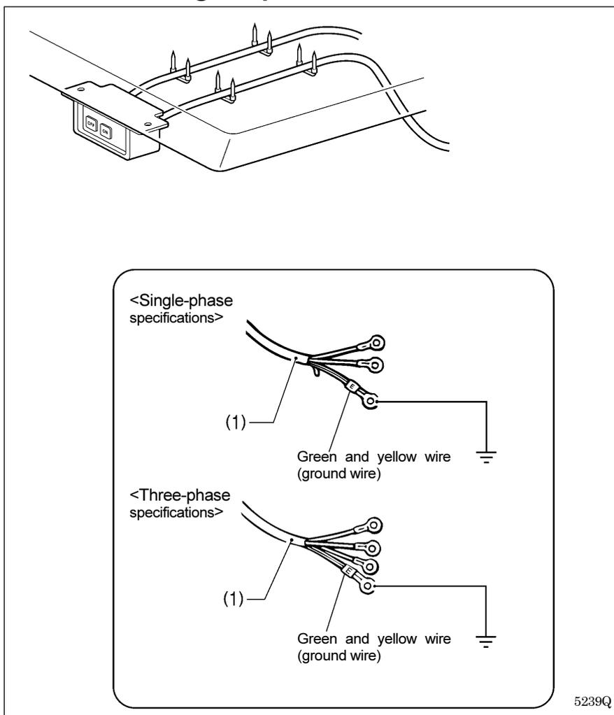
1. Attach an appropriate plug to the power cord (1). (The green and yellow wire is the ground wire.)
