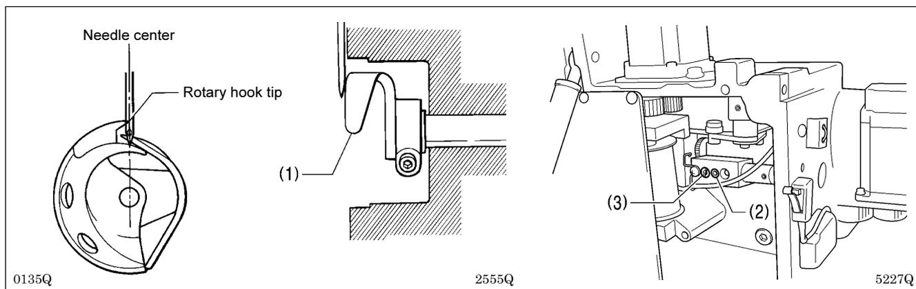
Turn the machine pulley to align the tip of the rotary hook with the center of the needle, and then loosen the set screw (2) and turn the eccentric shaft (3) to adjust so that the driver needle guard (1) is touching the needle.
