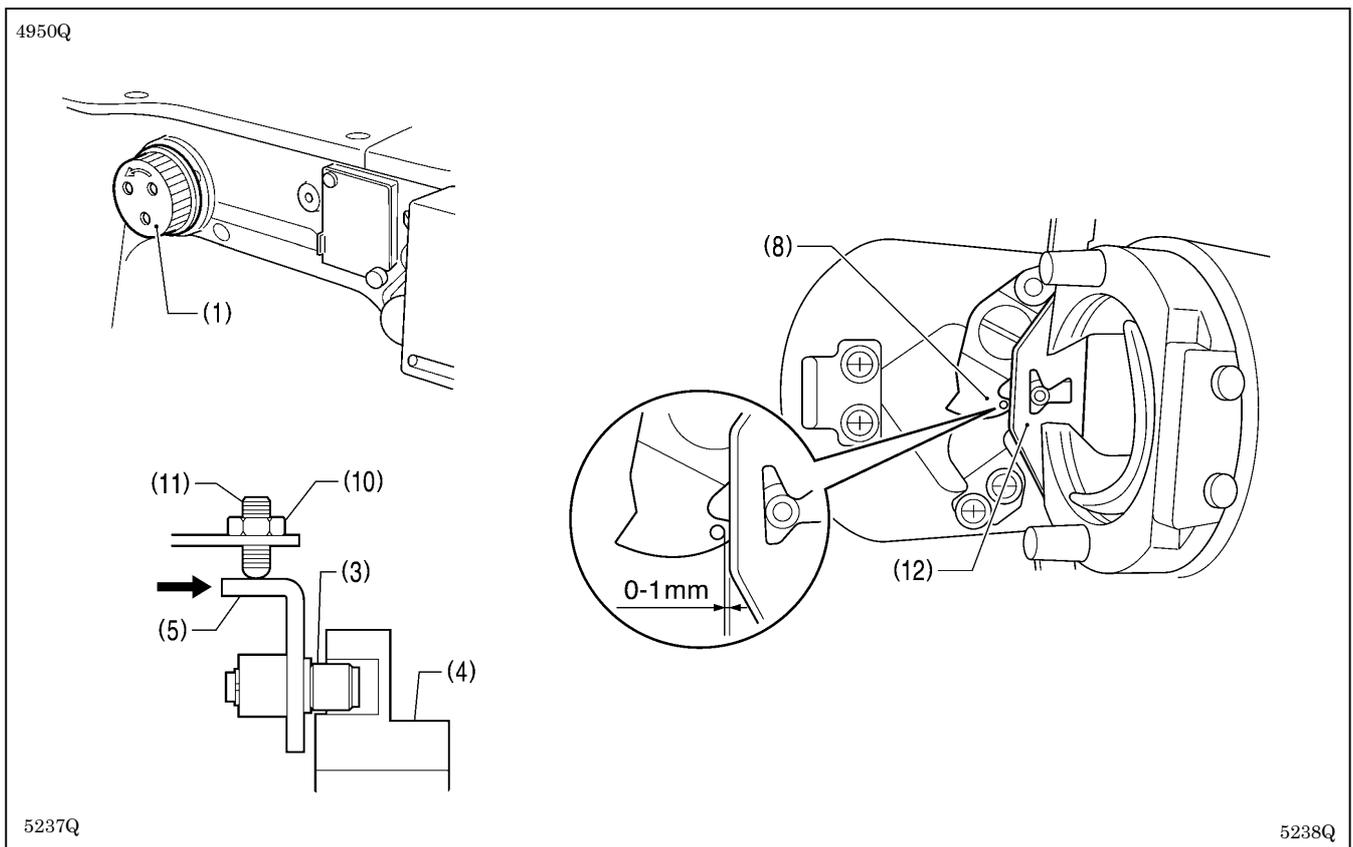
7. Turn the pulley (1) by hand to move the needle bar to its lowest position.
