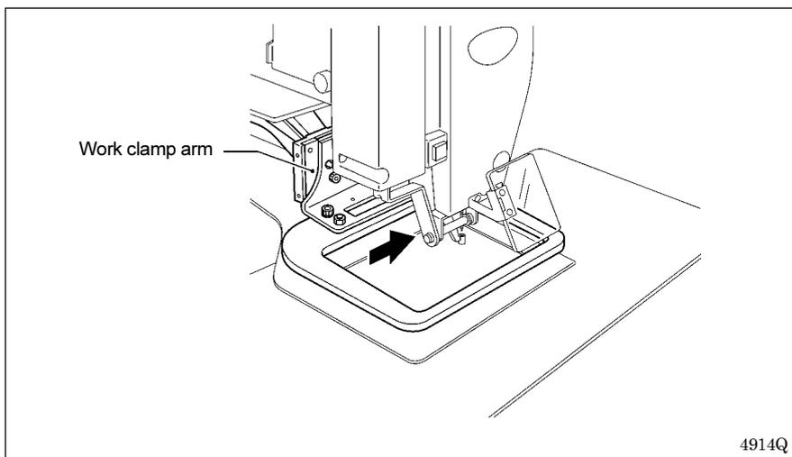
Move the work clamp arm all the way to the right when looking from the front of the sewing machine (the direction of the arrow in the illustration), and then gently tilt back the machine head.
