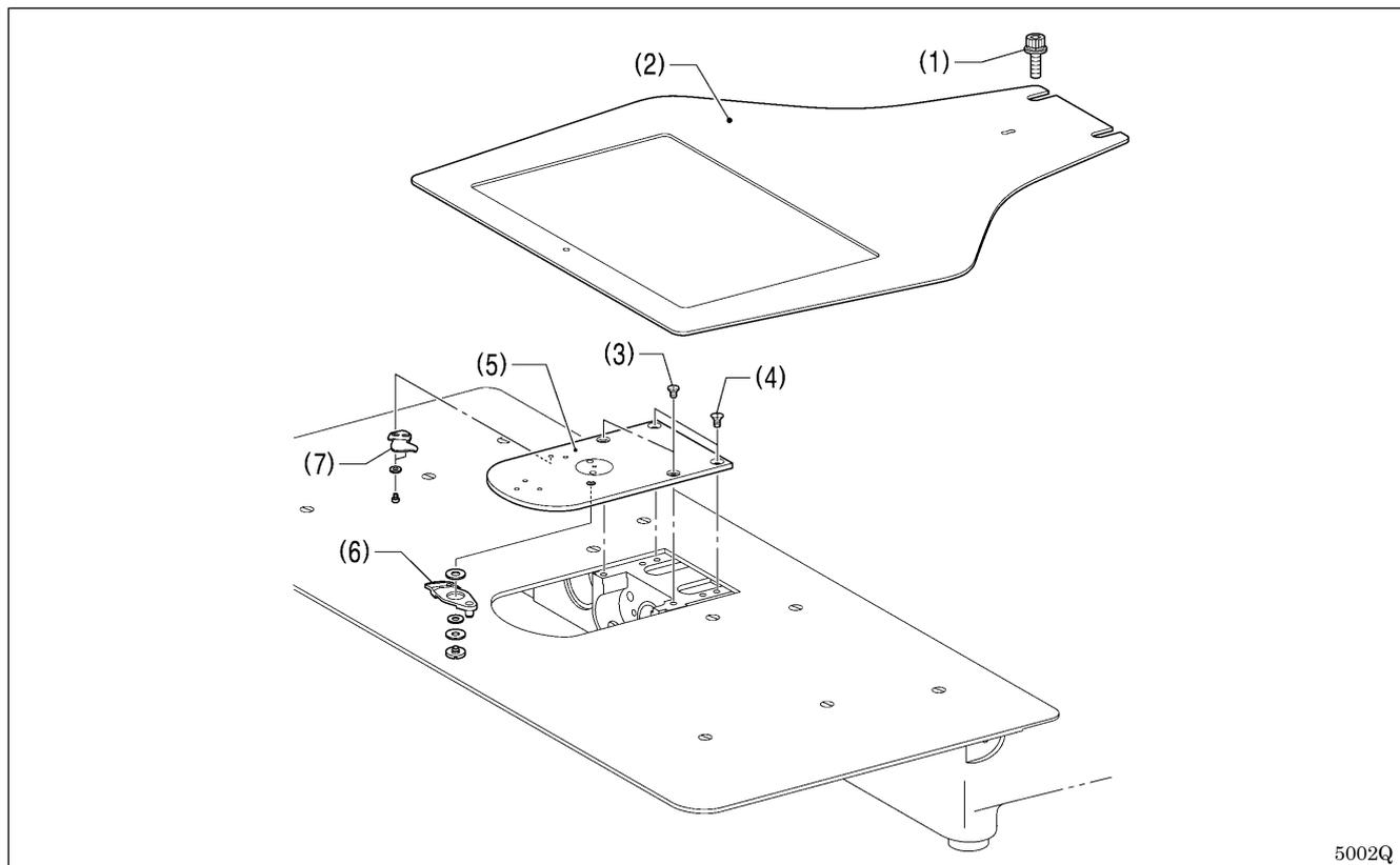
1. Loosen the two bolts (1) and then remove the feed plate (2).
